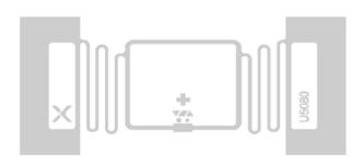
VersaMini FM features the FM051E chip. The "cutting performance retention" antenna design technology allows the same inlay to be adapted for labels ranging from 33-38mm in length and 13-18mm in width. It can not only be used as a normal label or liquid label, but also can be made into a flag suitable for metal packaging and a hanging label on iewelry through a deformed packaging design.
