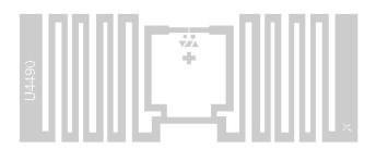
Spring M800 uses Impinj M830 chip. The antenna has been optimized and has good performance in the full frequency band (860-960 MHz). Through the test of the attached object scenario, the tag is suitable for various RFID tag applications, especially in clothing inventory management, logistics and other related fields.
