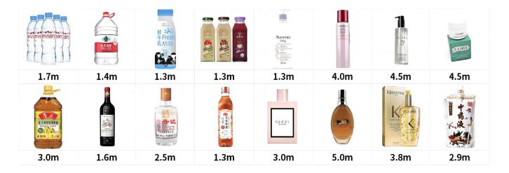
VersaMini recognition distance after being applied to the surface of a wide range of liquid products (tested on a C72 Handheld RFID Reader)
